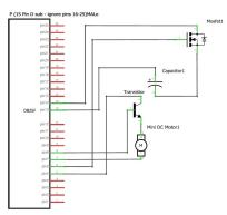
Figure : Wiring diagram for the Small debris Collector
