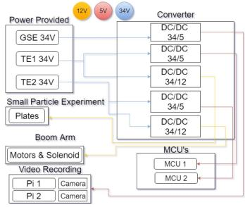
Figure : Functional Block Diagram for Power
