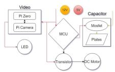
Figure : Functional block diagram for the Small debris Collector
