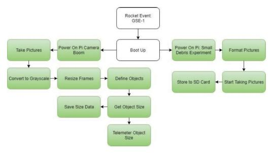
Figure : Software flow chart of Pi cameras.
