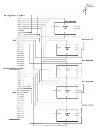
Figure : Electronics diagram for step-down converters
